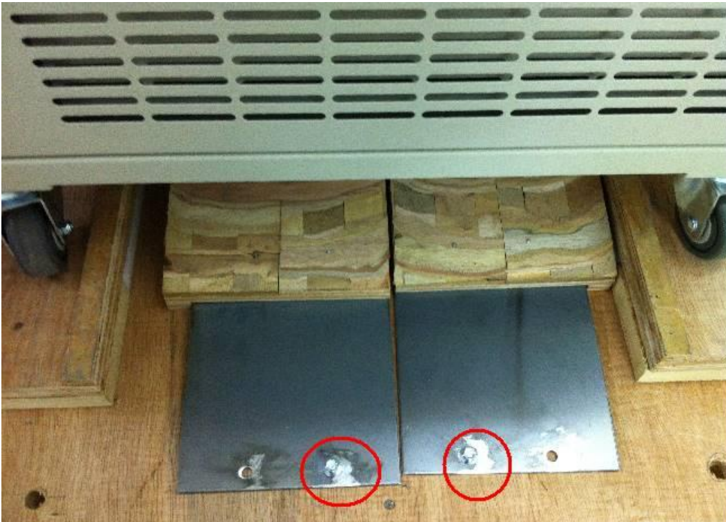
Step 6: Unscrew the screws fastening the slide boards on the pallet
