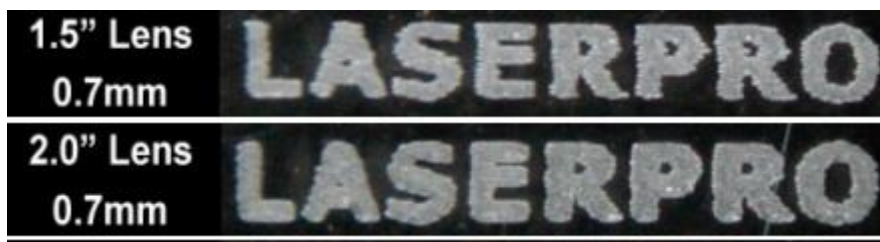
Cutting edges achieved with the different lenses
