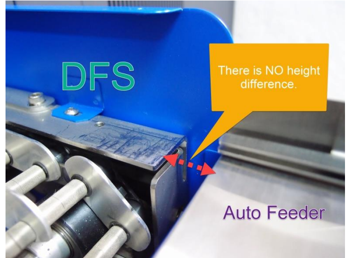
After Adjustment (there is no height difference)
