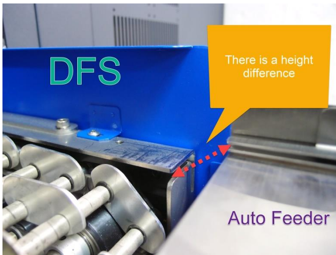
Before Adjustment (there is a height difference)
