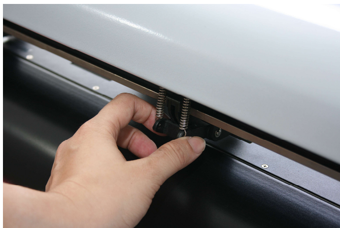
Figure 4-3 correct way to move pinch rollers
