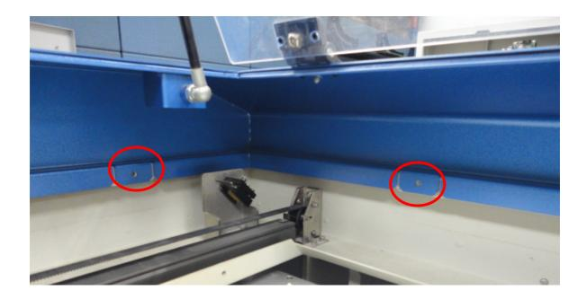
2. Disconnect circles cables show in below picture(blue circles) and Loosen four screws (red circles) for the fixing of Control Panel and you can replace the Control panel
