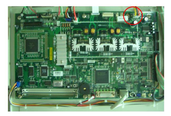
4. Loosen five screws to remove the power board (see picture below)
